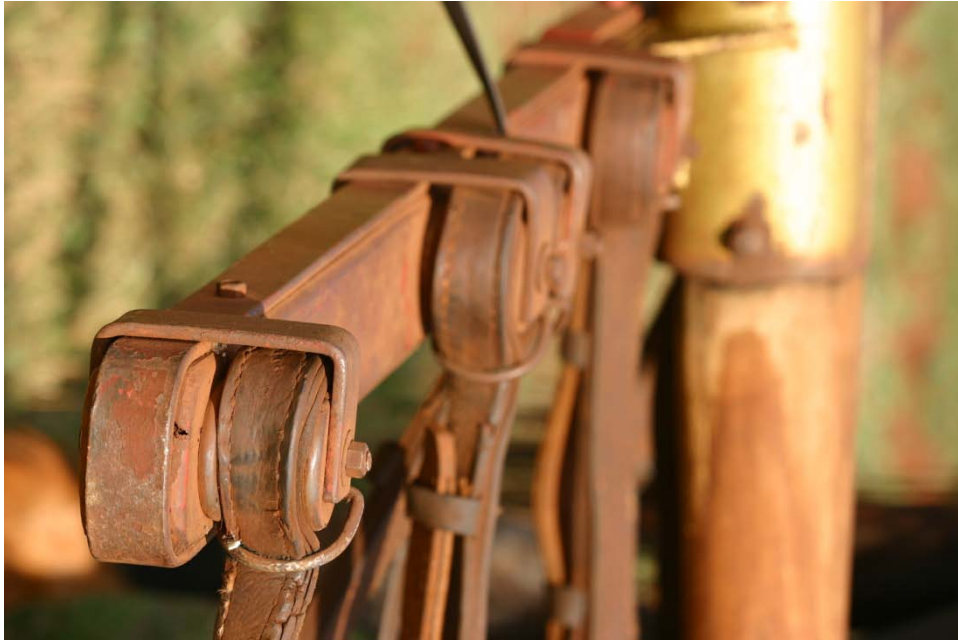
Picture 4: Supported by this diagonal, a horizontal bar measuring the four horses receives the fixation of the pulley system that maintains the reins connected. The leader moves the four horses by the two reins in which he sustains in each hand.
